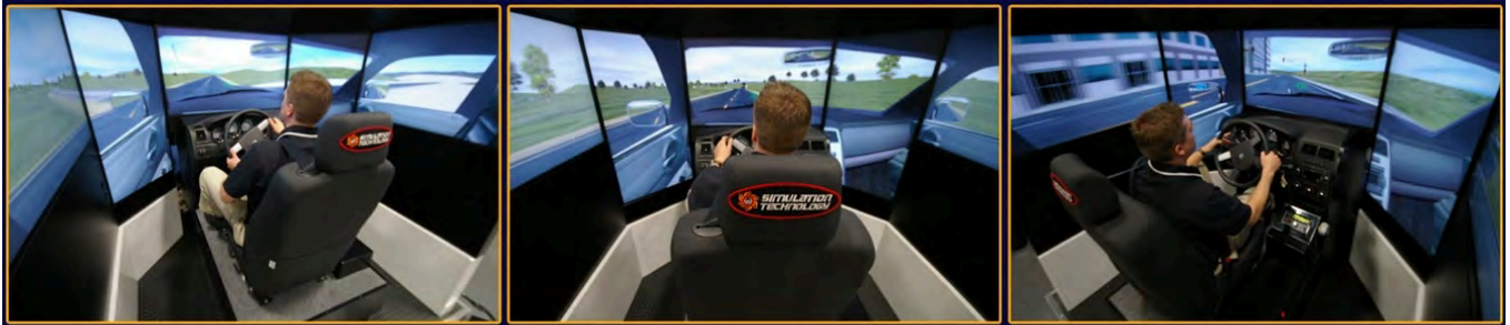
The 2010 Dodge Charger LE Driving Simulation System from Simulation Technology: 230+ degree FOV, real vehicle cockpits, real OEM parts for IP and siren/flasher controls, run on the authentic J1939 CAN-bus communications....all run on one computer.
